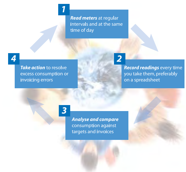
Figure 1 Reading meters for energy management
