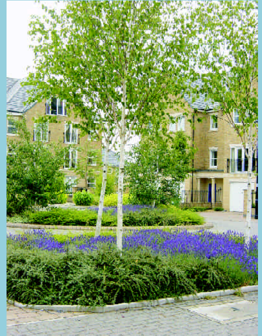
A high quality landscape scheme. Trees should have a girth of 14-16 cm and should be adequately staked to prevent vandalism - Southampton
