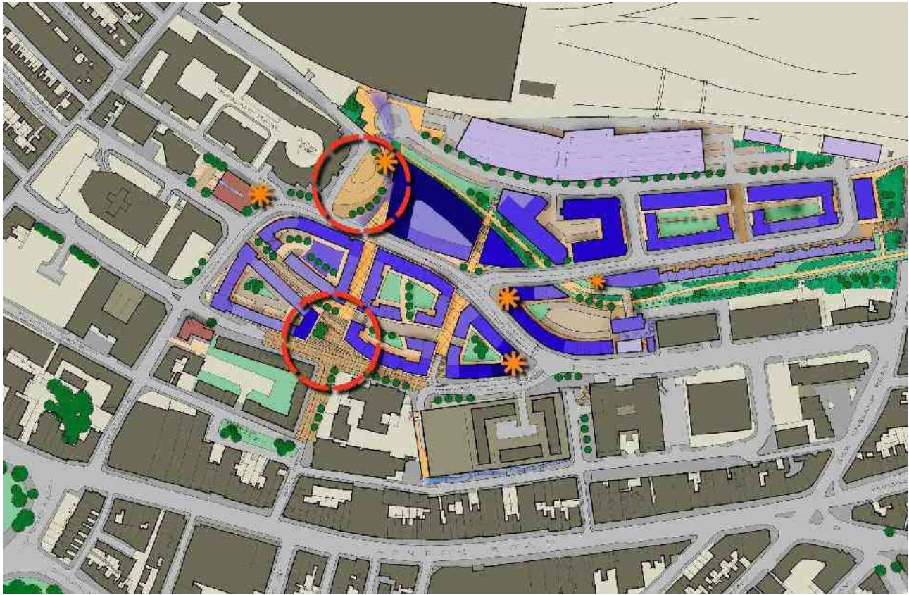
Brighton Goods Yard redevelopment. Linkages strengthened between many destinations either side of the site. Pedestrians have priority on the majority of links across the site. Impact of the new highways scheme is kept to a minimum.
