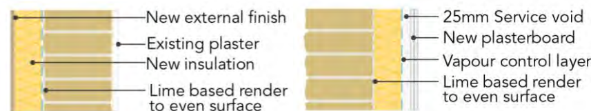
Externally insulated Stone Wall
