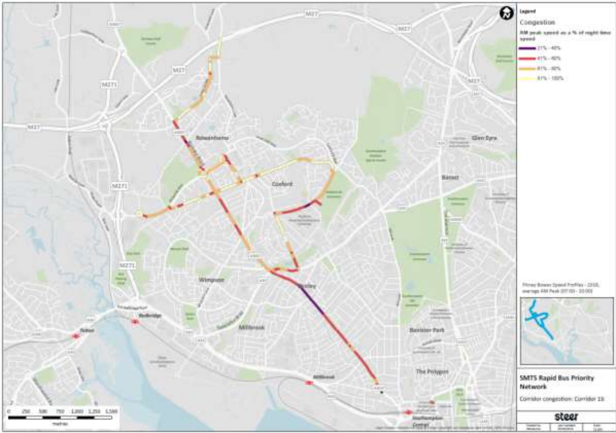
Figure 2.5 Example of Impact of Traffic Conditions on Speeds and Buses – Shirley Road
