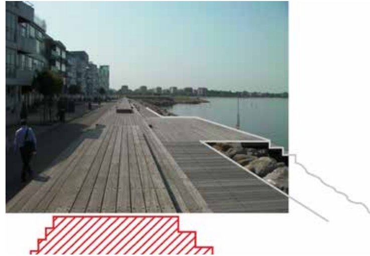
Integrating a 'flood wall' into waterfront development
