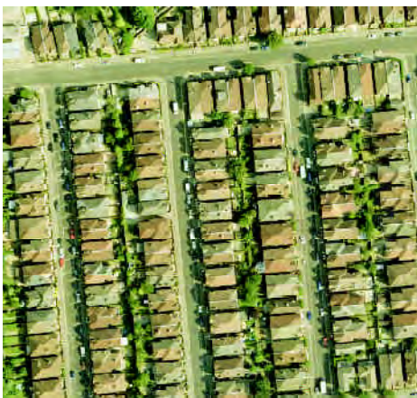
An aerial view of the above housing shows the 'grid-iron' pattern of development
