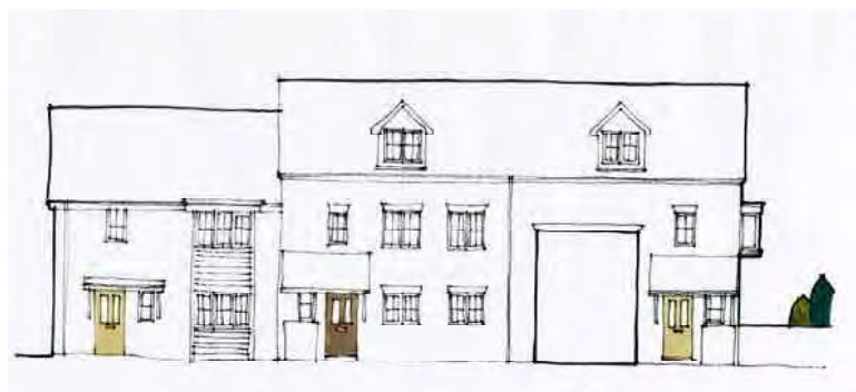
This archway is too high for its width and leaves a blank wall above the opening that is visually 'heavy'
