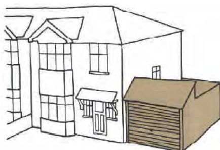
Good - An integrated garage design where the pitch of the roof reflects that of the existing house and integrates the extension by continuing the roof from the garage over the existing front door to provide a porch.
