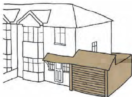
Good - An integrated garage design where the pitch of the roof reflects that of the existing house and integrates the extension by continuing the roof from the garage over the existing front door to provide a porch.
