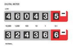
Reading a single register digital meter.
